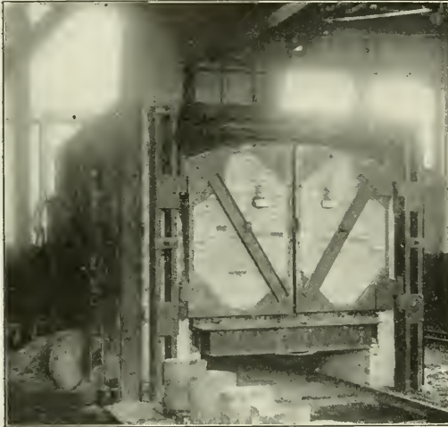
Oil Burner Type Annealing Oven.
